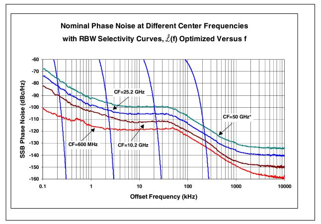
\*Unlike the other curves, which are measured results from the measurement of excellent sources, the CF = 50 GHz curve is the predicted, not observed, phase noise, computed from the 25.2 GHz observation. See the footnotes in the Frequency Stability section for the details of phase noise performance versus center frequency.
