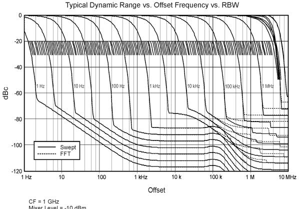
Mixer Level = -10 dBm Only 2/decade of the 24/decade RBW are shown fully RBWs ≤ 1 kHz shown with phase noise optimized for fm < 50 kHz RBWs ≥ 3 kHz shown with phase noise optimized for fm > 50 kHz
