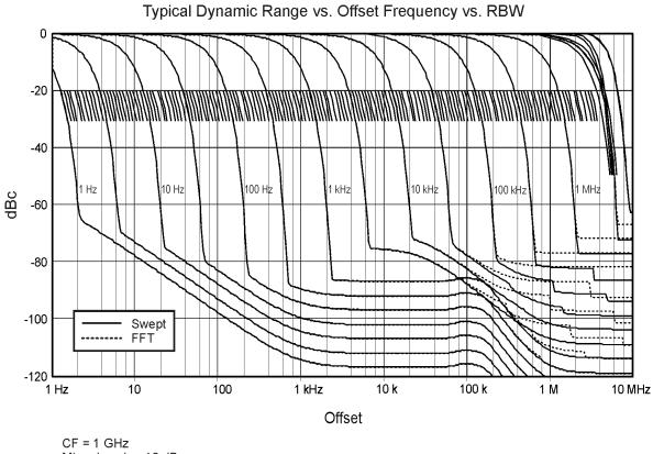
CF = 1 GHz Mixer Level = -10 dBm Only 2/decade of the 24/decade RBW are shown fully RBWs  $\leq$  1 kHz shown with phase noise optimized for fm < 50 kHz RBWs  $\geq$  3 kHz shown with phase noise optimized for fm > 50 kHz
